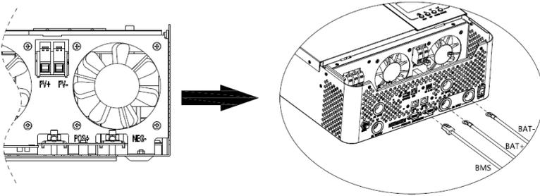
4. The other end of RJ45 insert to battery communication port(RS485 or CAN).
