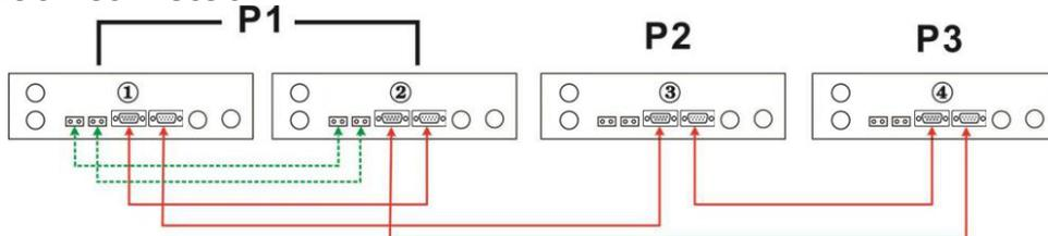
Two inverters in two phases and only one inverter for the remaining phase:
