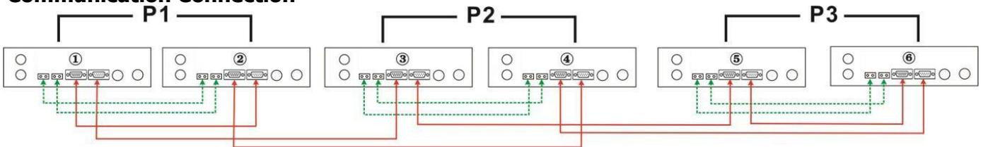
Three inverters in one phase, two inverters in second phase and one inverter for the third phase:
