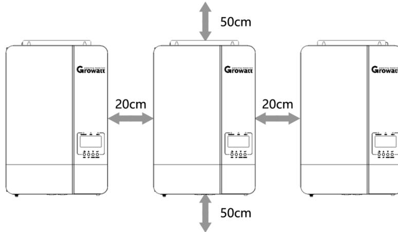
**Note:** For proper air circulation to dissipate heat, allow a clearance of approx. 20cm to the side and approx. 50 cm above and below the unit. Be sure to install each unit in the same level.
