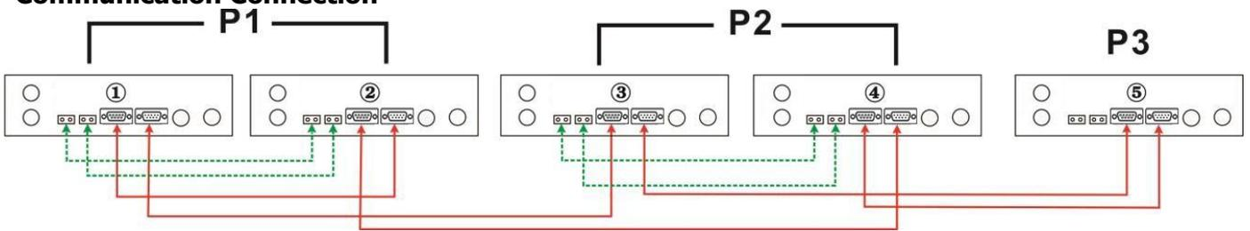
Three inverters in one phase and only one inverter for the remaining two phases:
