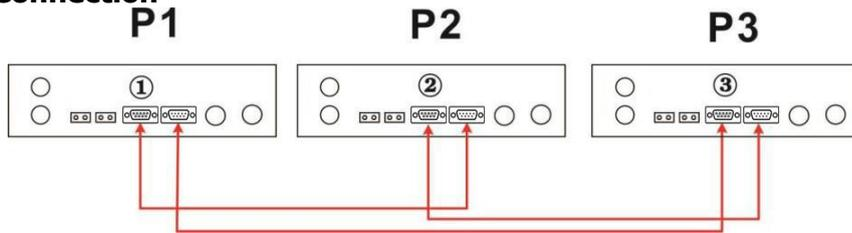
Two inverters in one phase and only one inverter for the remaining phases:
